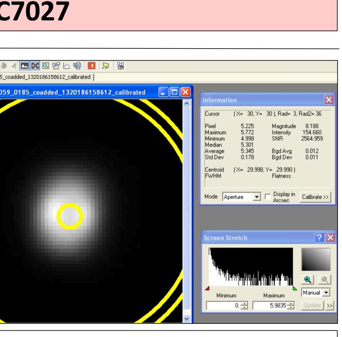
(Above) Intensity measures were made using MaxIm DL. An Aperture radius of 3 pixels (~2.4") was selected since, 1) the images themselves could not be precisely aligned, and 2) the measured FWHM resolution of the FORCAST camera across the channels is ~3.6-to-
