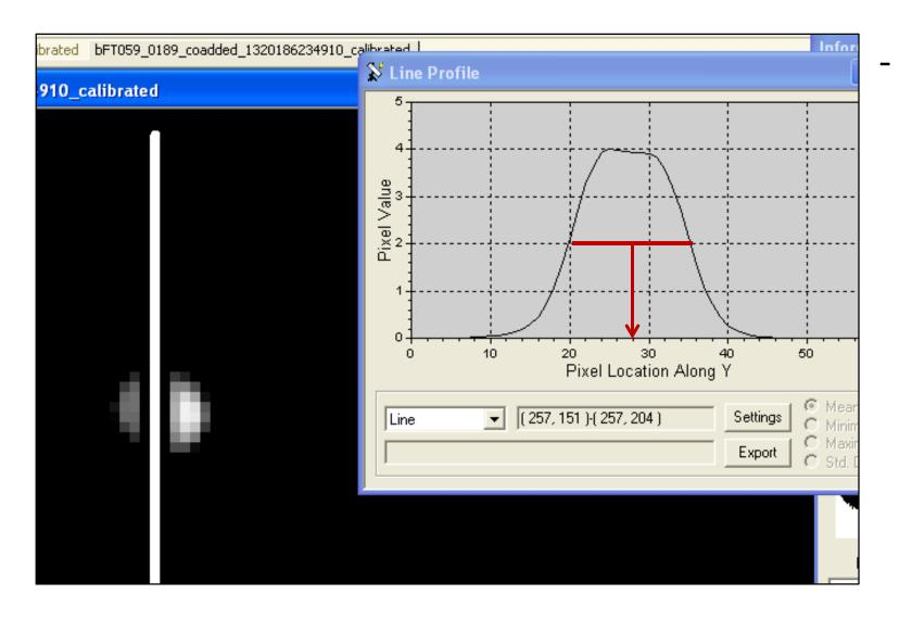
SOFIA images did not contain world coordinate data in the headers, making it a image challenge to align images for further analysis. Vertical slices were taken across NGC7027 to establish the central lane, and the center pixel at Full-Width-Half-Max (FWHM) of the profile was established as NGC7027's center. (See image left)
