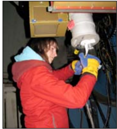
Above: Inga Saathoff filling up the dewar of the 0.9 meter Telescope. The project has received a total of 4 nights observing at Kitt Peak National Observatory through the RBSE – TOPS Program.
